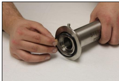
Photo 2.1: Outer Ring Insertion
