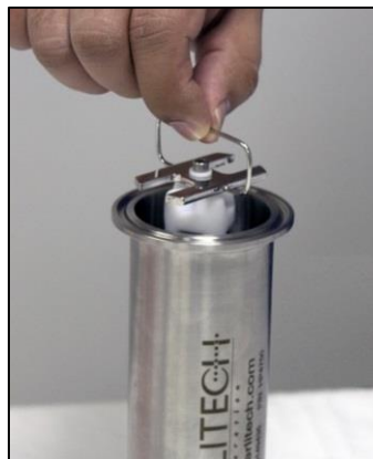
Photo 2.8a: Stir Bar Insertion
