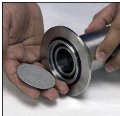
Photo 2.4: Membrane Support Disk Insertion
