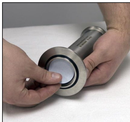
Photo 2.3: Membrane Filter Insertion
