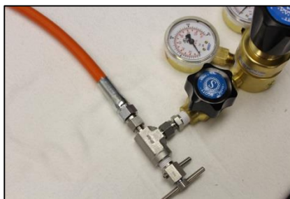
Photo 2.13: Pressure Regulator Connection
