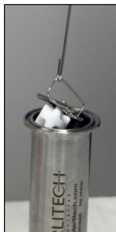
Photo 2.8b: Stir bar Insertion with stir bar retriever
