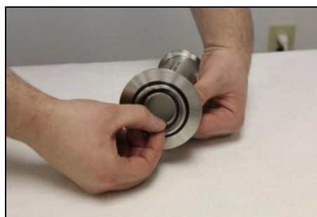
Photo 2.2: Inner Ring Insertion
