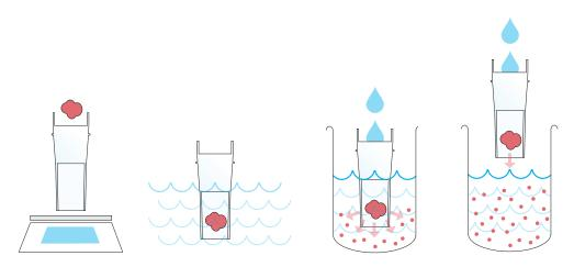
The unique, patented Hydrocap filter contains the sample from the initial weighing, through hydrolysis to final extraction; avoiding sample transfer errors. It is a fully automated system that performs addition of acid, heating, boiling, rinsing and draining.
