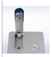
Micro-volume UV/VIS measurement is the method of choice if small sample amounts or if high absorption samples need to be measured. Only 1 µL of sample is required for reliable measurements. The pure sample is pipetted on the measurement surface and the arm is automatically locked to a precisely defined pathlength. Measurement errors are avoided as the sample does not need to be diluted.
