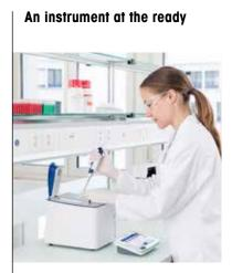
FastTrack UV/VIS technology guarantees that the instrument is ready at all times. No warm up time is needed for the Xenon flash lamp to reach stability, which speeds up measuring time. As the lamp is only used for real measurements, its lifetime is greatly increased.
