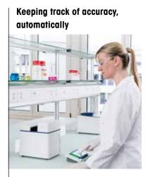
The CertiRef<sup>™</sup> performs all tests required in the UV5Bio to comply with the Ph.Eur. or USP pharmacopoeia. It automatically verifies the resolution, photometric and wavelength accuracy, and stray light. Certified reference materials traceable to NIST are used and a comprehensive report documents all results. Performance verification has never been so easy, efficient and secure. High performance, low maintenance
