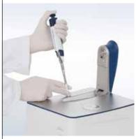
The UV5Nano is two instruments in one for micro-volume and cuvette based measurements. Once the arm is at 90 degrees position the measurement surface can be easily accessed with a pipette from either the left or the right side. The curved lid on top of the instrument allows convenient positioning of the operator's hand to securely guide the pipette tip.
