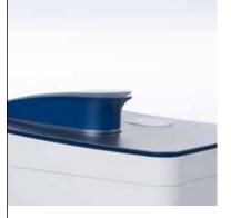
LockPath<sup>™</sup> enables the measurement of wide concentration ranges from 6 to 15.000 ng/µL of dsDNA without further dilutions. This and measurement accomplishment within 2 seconds per pathlength saves a lot of precious time. The arm design effectively prevents drying out of sample during measurement, which stabilizes measurement repeatability.
