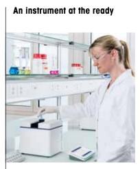
FastTrack UV/VIS technology guarantees that the instrument is ready at all times. No warm up time is needed for the Xenon flash lamp to reach stability, which speeds up measuring time. As the lamp is only used for real measurements, its lifetime is greatly increased.
