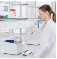
The UV5Nano combines two instruments in one for microvolume and cuvette based measurements. Once the arm is at a 90 degree position, the measurement surface can be easily accessed with a pipette from either the left or the right. The curved lid on top of the instrument allows convenient positioning of the operator's hand to securely guide the pipette tip.
