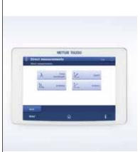
Spectrum scans, fixed wavelength absorption measurements, quantification with calibration curves or kinetic analyses are ready to use as direct measurements: Simply enter parameters, define the preferred workflow, store as a shortcut, and start the measurement with One Click.
