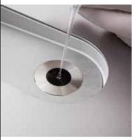
Micro-volume UV/VIS measurement is the method of choice when measuring either small sample amounts or high absorption samples. Only 1  $\mu$ L of sample is required for reliable measurements. The pure sample is pipetted on the measuring surface and the arm is locked automatically to a precisely defined pathlength. Measurement errors are avoided, as the sample does not need to be diluted.
