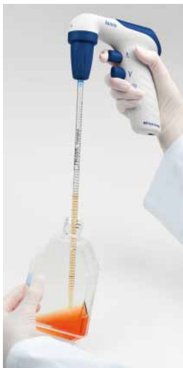
0.2 micron disc filter protects from contamination
